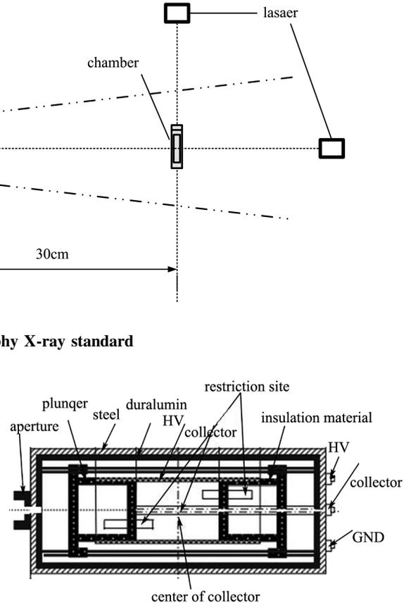
Fig. 2 Cylindrical free air ionization chamber
