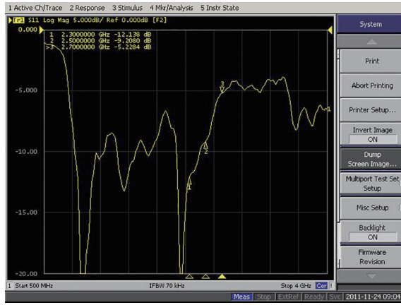
Fig. 10 The measured S_{11} curve
