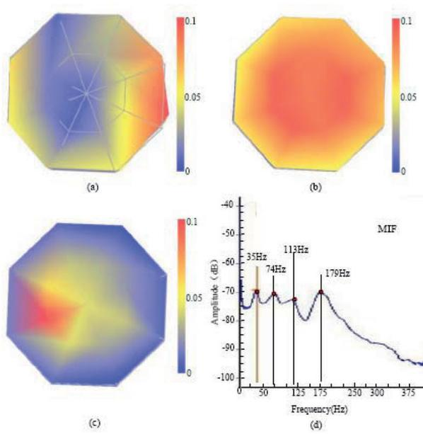
**Fig. 5 Modal Vibration Characteristics for Ap Landmines: ( A ) First-Order Vibration Mode, ( B ) Second-Order Vibration Mode, ( C ) Third-Order Vibration Mode, ( D ) Modal Indication Transfer Function**
