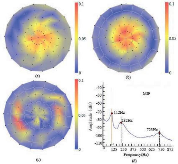
**Fig. 3 Modal Vibration Characteristics for Plastic Landmines: (A) First-Order Mode Shape, (B) Second-Order Mode Shape, (C) Third-Order Mode Shape, (D) Modal Indication Function**
