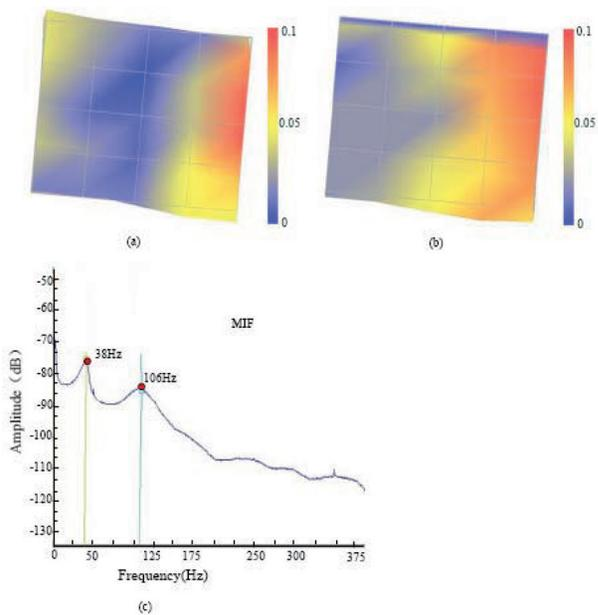
**Fig. 6 Modal vibration characteristics for bricks: ( a ) First-order vibration mode, ( b ) Second-order vibration mode, ( c ) Modal indication transfer function**
