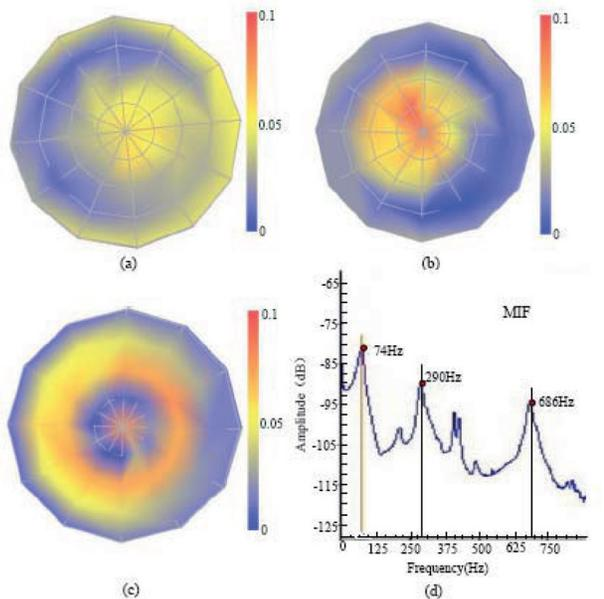
**Fig. 4 Modal Vibration Characteristics for Metal Landmines: (A) First-Order Vibration Mode, (B) Second-Order Vibration Mode, (C) Third-Order Vibration Mode, (D) Modal Indication Transfer Function**
