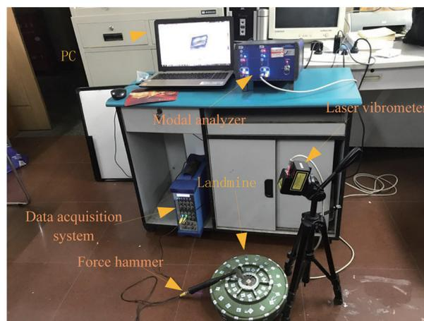
Fig. 2 Multi-Modal Vibration Mode Testing System for Landmines
