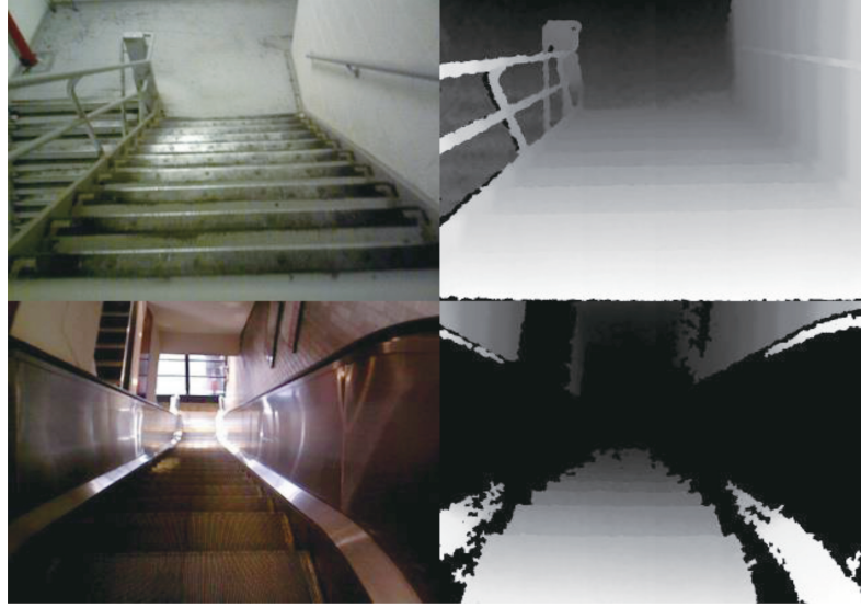
Fig. 1 Examples of the RGB image and the depth image of the downstairs stationary stairway dataset are shown on the top-left and top-right corners, respectively. Examples of the RGB image and the depth image of the downstairs escalator stairway dataset are shown on the down-left and down-right corners, respectively. An obvious shift between the two data distributions can be observed.
