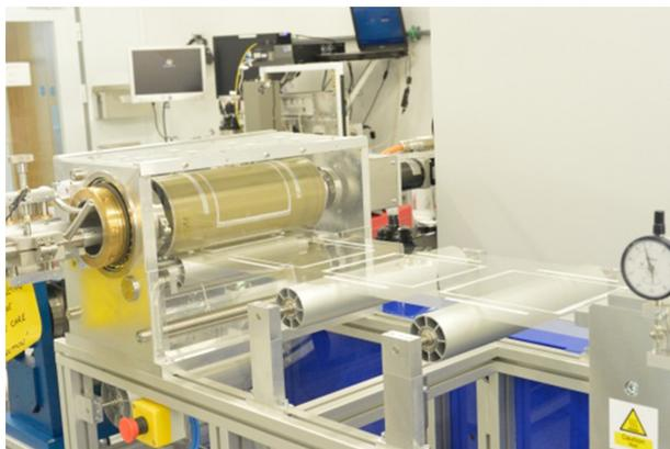
**Fig. 4 Rotary screen printed adhesive annulus**
