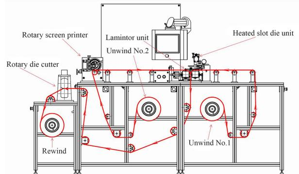
Fig. 2 Roll to roll framework showing the direction (indicated by the bold arrowed red lines) of the web
