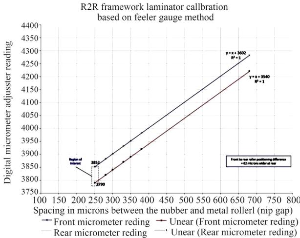
Fig. 7 R2R laminator gap calibration graph
