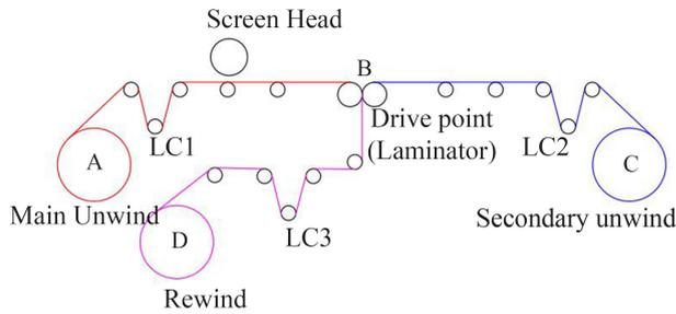
**Fig. 3 Film tension control system**
