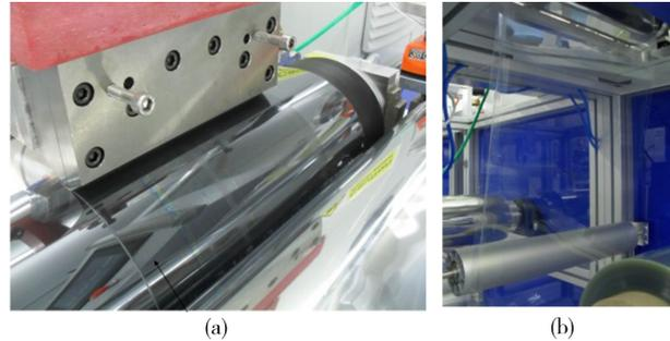
**Fig. 6 (a) Liquid crystal coating using slot-die
