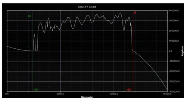
**Fig. 5 Surface profile of rotary screen printed adhesive annulus section**
