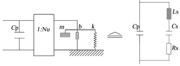
Fig. 3 Equivalent circuit of a CMUT cell
