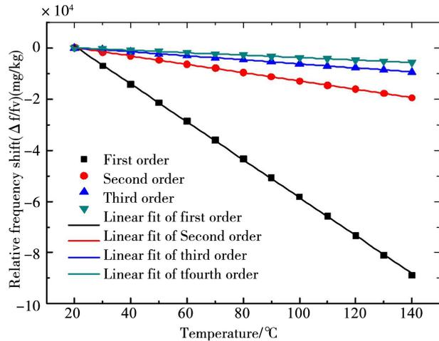
**Fig. 4** Relative frequency shift VS temperature under different vibration modes of the membrane.
