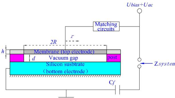
**Fig. 1** Schematic of a CMUT cell for temperature measurement
