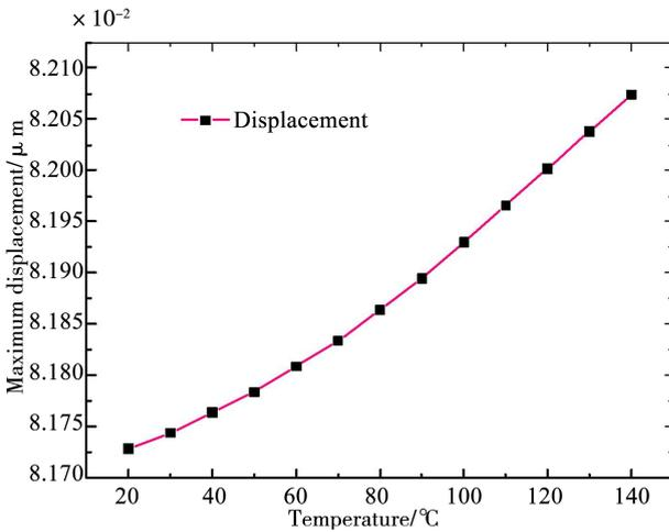
**Fig. 6** Variation of the maximum deflection of the membrane with respect to temperature at a bias voltage 80% of the  $U_{colla}$ .
