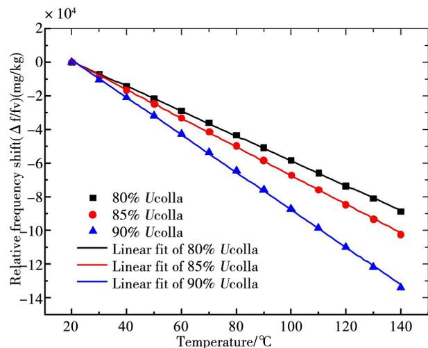
**Fig. 5** Relative frequency shift VS temperature at different bias voltages.
