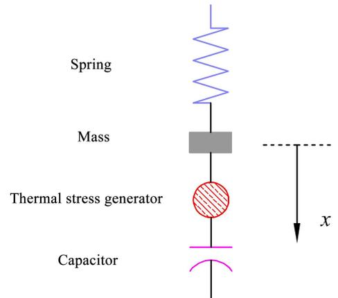
**Fig. 2** a lumped electro-mechanical-thermal model for a CMUT cell
